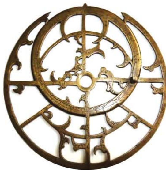
Fig. 16. Rete in the Moscow astrolabe of 1587 © The State Museum of Oriental Art, Moscow
