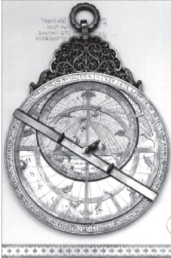
Fig. 1. The Gurmukhi Astrolabe, the front. The alidade is wrongly attached to the front. It should have been fixed on the back
