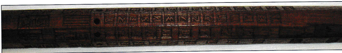
Fig. 7 Column Dial (detail), private collection in Brussels; the scale facing the reader is filled with carved Nagari numerals from 1-14. The names of the months are written above the scales. Photo by S. R. Sarma.
