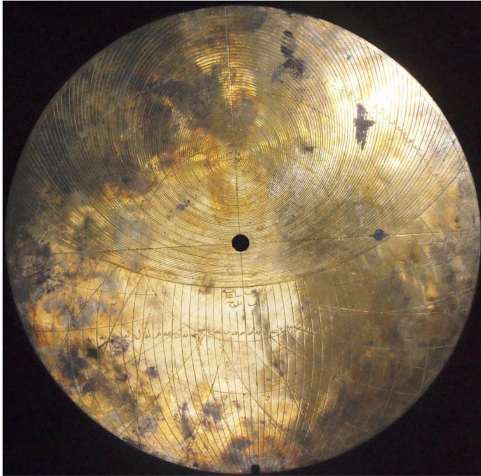
Fig. 4 The Plate for Lahore at the Latitude of 32 degrees
