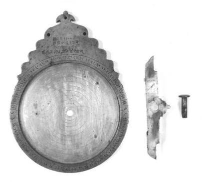
Figure 5: The inner side of the body with an empty grid; alidade and pin.
